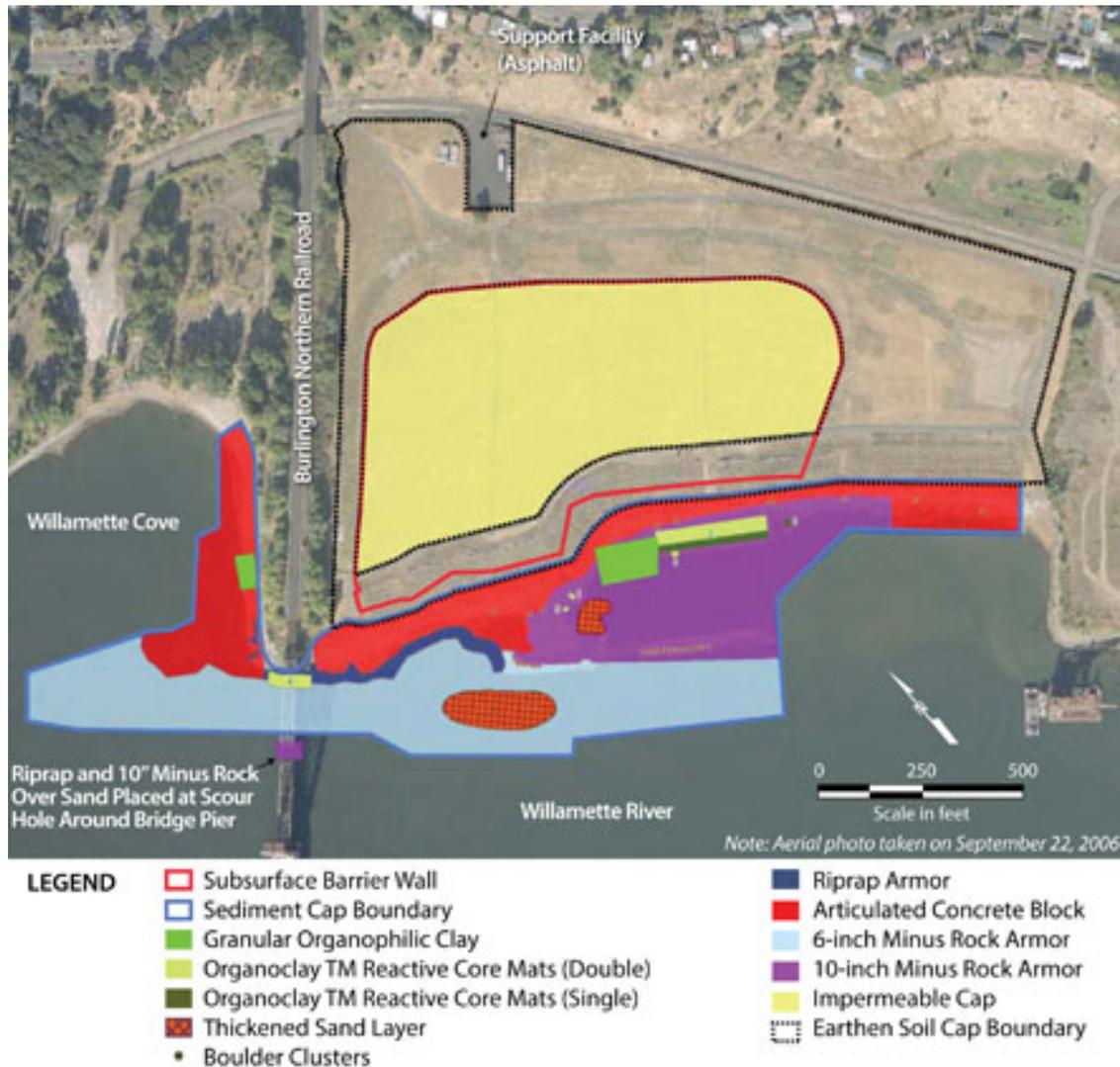
**Figure 1.** Aerial schematic of multi-component containment system operating at the McCormick & Baxter site.
