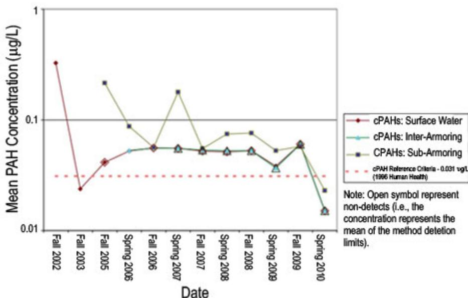
**Figure 6.** Mean concentrations for total cPAH in surface water, inter-armor water (collected within the rock armor), and sub-armor (sand cap) water of the sediment cap at the McCormick & Baxter site.
