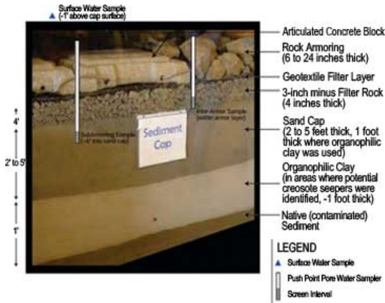
**Figure 3.** Cross-section of sediment cap installed at the McCormick & Baxter site.
