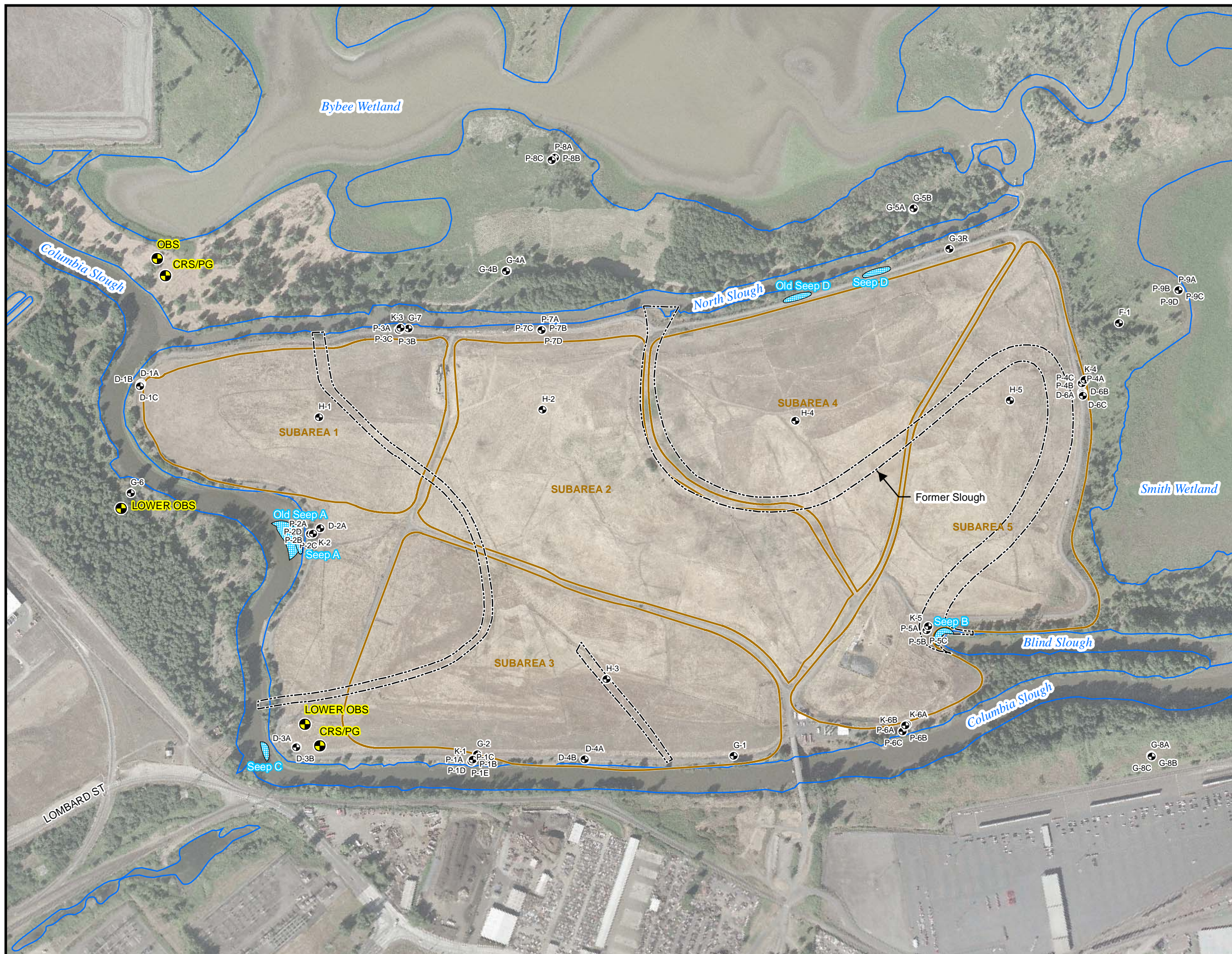
Figure 8 Proposed Monitoring Well Locations St. John's Landfill
