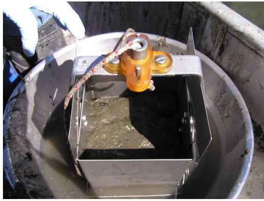
Eckman dredge sampler used for deep water locations
