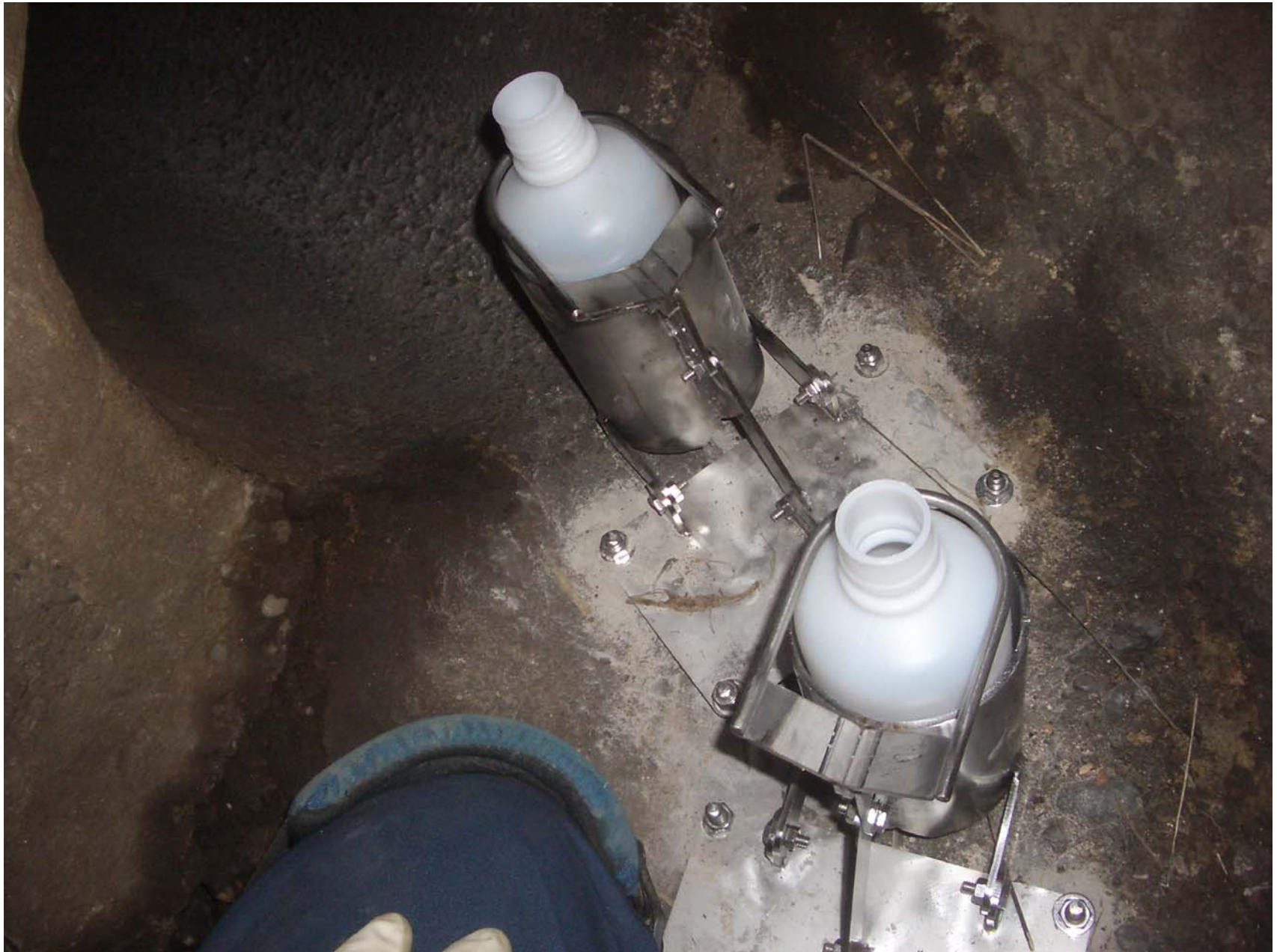
Figure 2-2 Photo of Sediment Trap Round 3A Stormwater Field Sampling Plan
