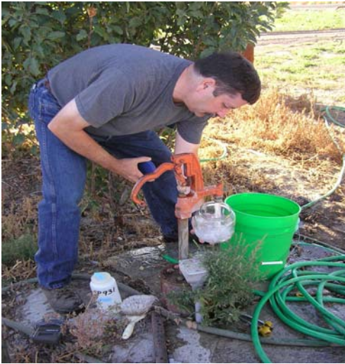
A water quality monitoring specialist collects a pesticide sample from a Northern Malheur County Groundwater Management Area well spigot.
