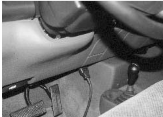
The OBD test consists of a scan tool that plugs directly into the vehicle's computer, giving an instant reading on the status of the emission systems.
